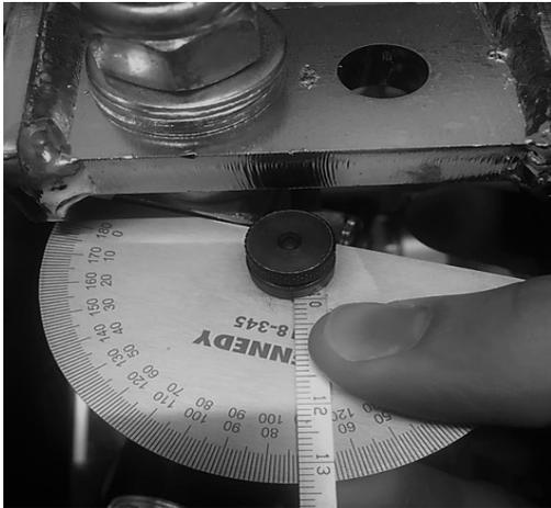
Rotate clevis mount 17 degrees clockwise.
